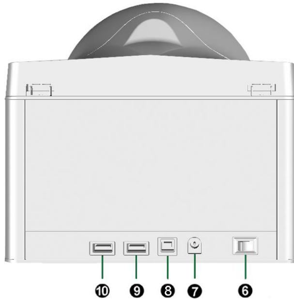
6. **Power Switch:** Use this to turn the scanner ON or OFF.
