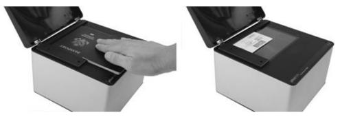
4. The scanner starts to scan immediately. After the scanning process is completed, the scanner will beep once and the scan indicator will blink once. The scanned image will display on the screen.
