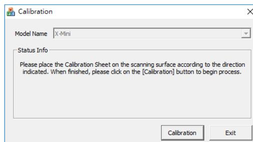
Place the special calibration sheet into the scanner with the printed side up, then click **Calibration** button.
