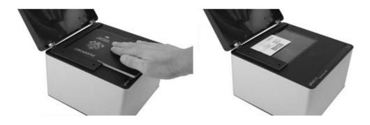
When you're scanning the passport, please gently press the passport binding to guarantee the minimum space between the to-be-scanned page and the scanner glass.
