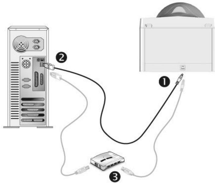
1. Plug the square end of the included USB cable to the USB port at the rear of the scanner.
