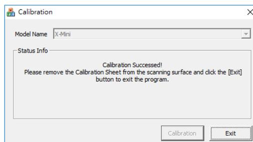
After the calibration is completed, please remove the calibration sheet then click **Exit** button.
