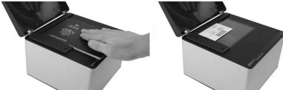
4. The scanner starts to scan immediately. After the scanning process is completed, the scanner will beep once and the scan indicator will blink once. The scanned image will display on the screen.
