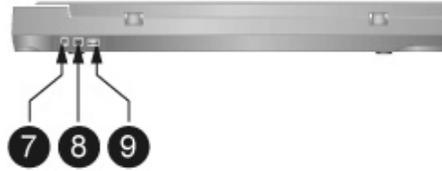
7. **POWER RECEPTOR**— Connects the scanner to a standard AC power outlet by the AC adapter included.
