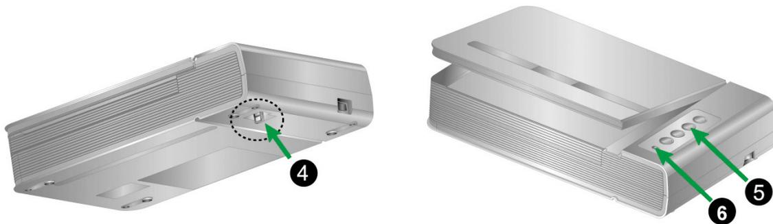
4. **Scanner Lock:** It holds your scanner head in place during transportation.
