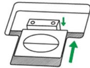
**Always Unlock** is for scanning on a surface that is not firm, unstable or too soft. Furthermore, if you place your scanner on a long-term position, you can also keep your scanner lock in this status.
