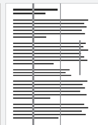
Gray Line Defect
