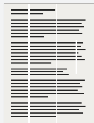
White Line Defect
