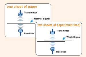
The ultrasonic sensor detects the double feeding of original documents during scanning. The ultrasonic function can be turned off for the purpose of intentional double-feeds such as taped receipt or sticky notes. This innovative design prevents double feeding and effectively scans documents of different weights or thickness. Thanks to double-feed prevention, optimum reliability is assured even when scanning high volumes of documents.
