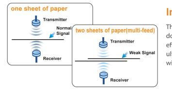
The ultrasonic sensor detects double feeding of original documents during scanning, and prevents double feeding and effectively scans documents of different weights or thickness. The ultrasonic function can be turned off when scanning document with labels, sticky notes, or taped receipts.
